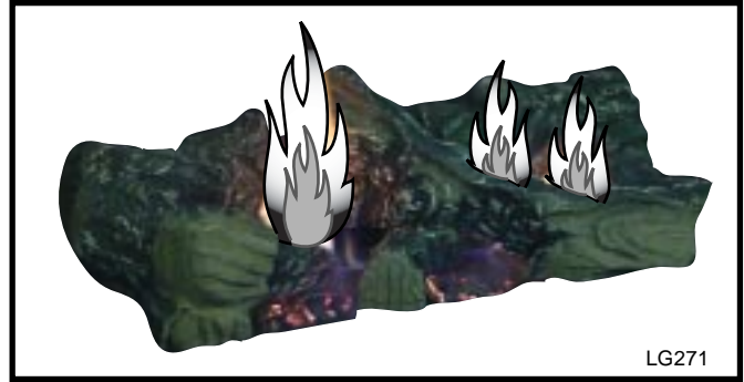
Fig. 45 Correct burner flame appearance for 33BDVR.
